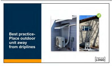
When needed, outdoor units should be installed with drip caps or shields.
