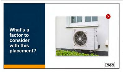
In colder climates, defrost cycle and full power operations occur frequently and run at Locate outdoor units where noise will not disturb occupants higher decibels than typical operations
